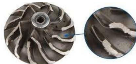
Figure: Failures of Compressor
